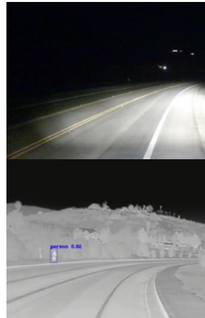
Figure 16: FLIR thermal sensors can classify pedestrians at distances four times farther than typical headlights.
