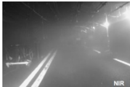
Figure 9. Example images recorded in fog tunnel with thermal (LWIR), visible RGB, short-wave (SWIR), and near (NIR) cameras. Copyright SIA Vision 2016
