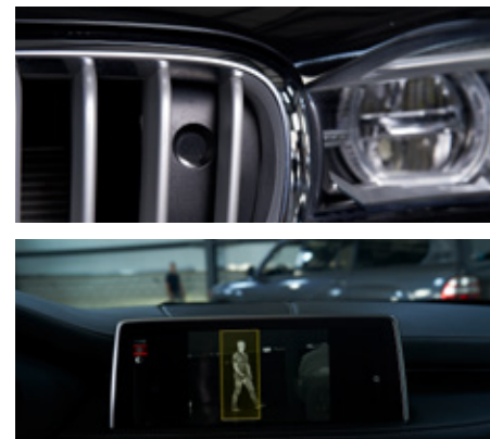
Figure 14: A grill-mounted FLIR thermal sensor integrated by Veoneer provides thermal vision for the BMW X5.
